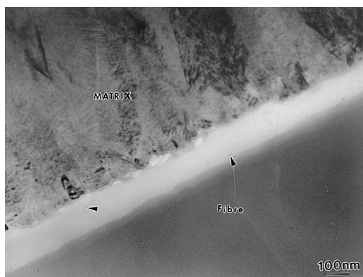
Fig. 3. TEM image of non-implanted zone of SiC/SiC composite – Interface.
